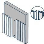
2. Install the second wall panel by placing the long connecting flap over the shorter flap.
