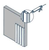
1. Install the first panel, and use construction glue to fix to place.
