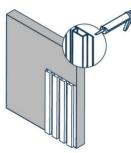
1. Install the first panel, and use construction glue to fix to place.
